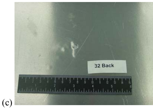
Figure D30. Sample 32 Views of Rear Wall Front (a & b) and Back (c) Faces after Hypervelocity Impact.
