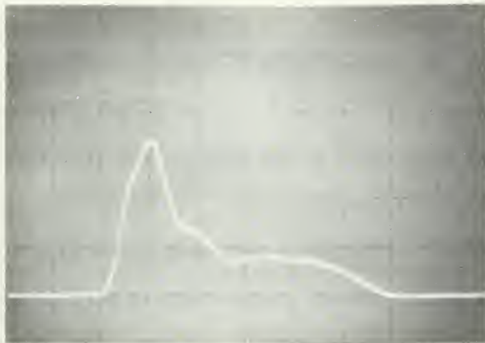
(a) Detected RF Envelope Using Sample No. 2. Horizontal Scale = 5 nsec/Division
