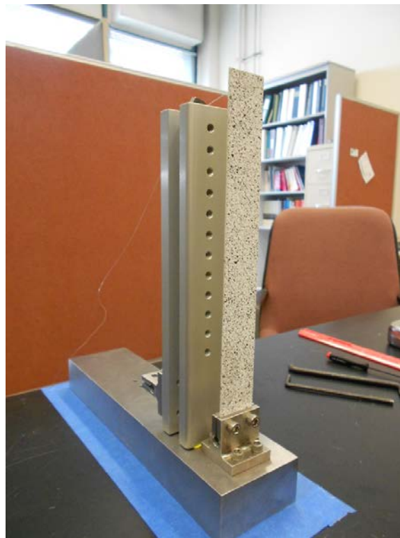
Figure 8. Image of cantilever testing apparatus
