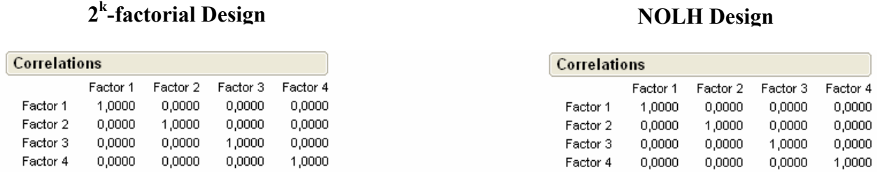
Figure 15. Comparison of the correlation matrices of a 2^k -factorial design and NOLH design.
