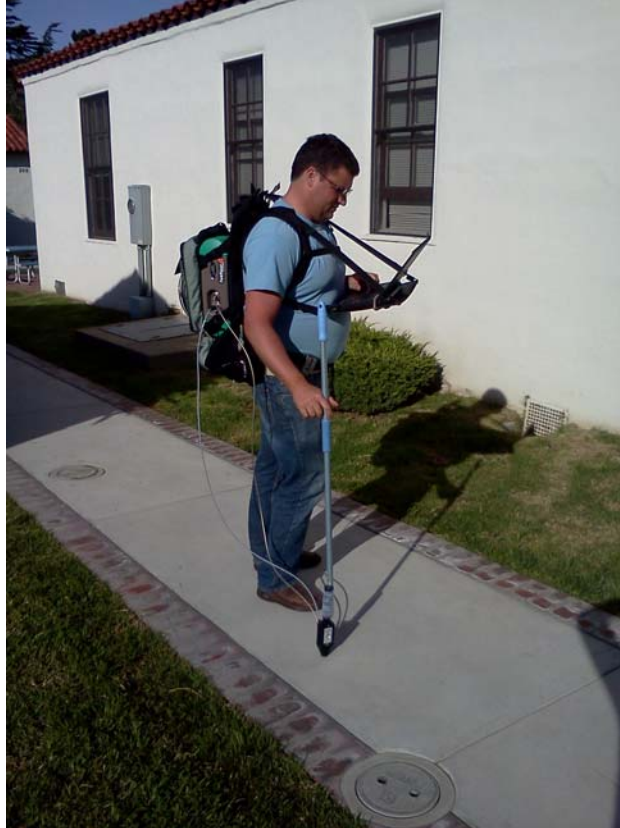
Figure 14. Photograph of typical ASD spectrometer configuration showing spectra being collected using a contact probe (with broom handle extension). FieldSpec 4 spectrometer unit is contained in the backpack. The fiber optic cable and power cable for the contact probe are seen.
