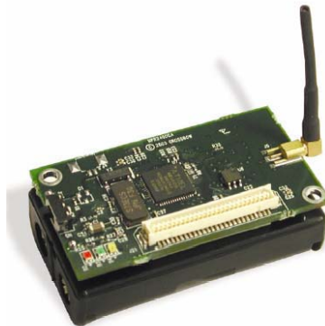
Figure 3. Actual MICAz Hardware. From Ref [19].
