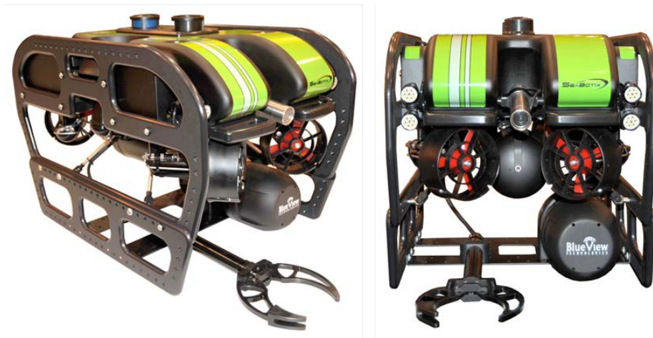
Figure 1. SeaBotix vLBV300 miniROV platform (From [15]) has been modified to allow tethered, autonomous operations.
