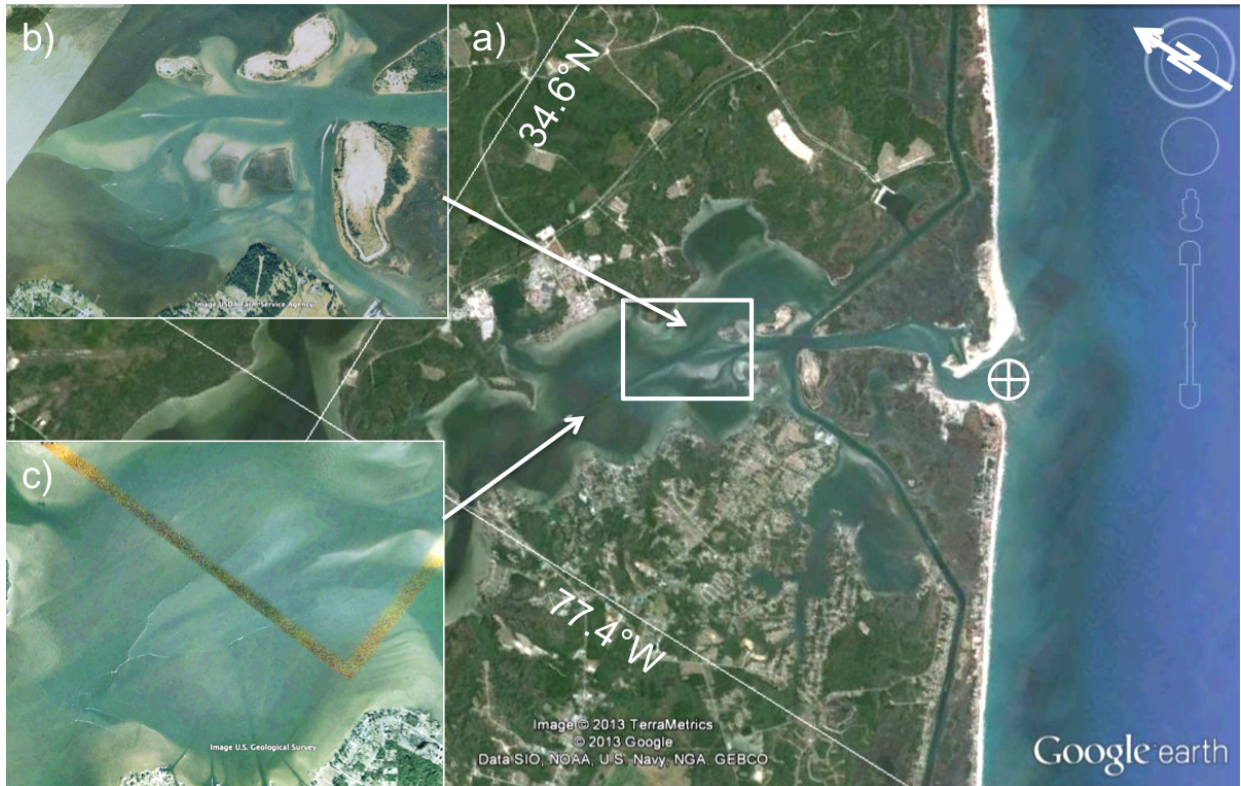
Figure 13. New River Estuary (NRE), North Carolina. (a) Latitude, longitude, and North references for the local 58^\circ RIVET axis rotation are labeled in white. Cross hairs at the mouth of the inlet show the local coordinate origin. (b) Close up of flood tidal intrusion in main tidal channel, showing clear ocean water displacing dark, turbid estuary water. (c) Close up of V-shaped surface convergence front farther up estuary. [From Google Earth , 2013].
