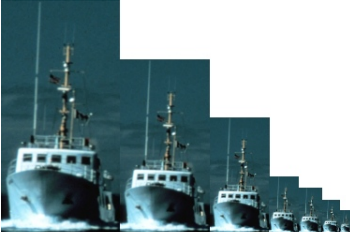
Figure 1. Example of a cropped ship image with the average pixel height of the evaluation set, and the subsequent 75, 50, 25, 20, 15 and 10 percent scales of the image, used to find probability of detection by range (after [5]).
