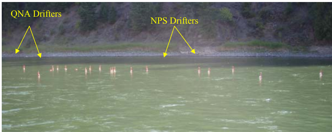
Fig. 4 Picture of river drifter deployment on the Kootenai River. QNA Drifters are pink balls and NPS drifters are pink rods. [1]
