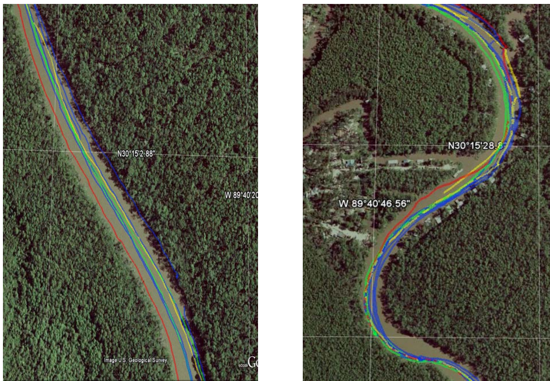
Fig. 5 Riverine Drifter Patterns over Six (6) Days Testing in West Pearl River
