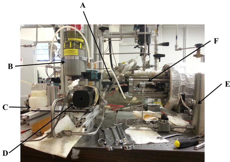
Figure 19 EMD injector setup: A) hydraulic piston, B) high pressure accumulator, C) spent hydraulic fluid, D) 1/2" ball valve, E) EMD injector, F) injector fuel tank
