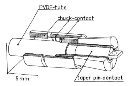
Figure 19. Piezoelectric Mechano-Electrical Transduction Mechanism [From 58]
