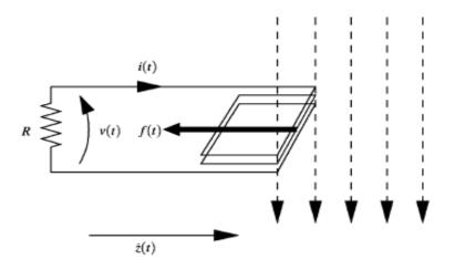
Figure 11. Electromagnetic Transduction Principle Operation [From 40]
