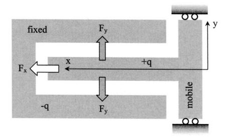
Figure 14. Single Axis Isolation Through Symmetry [From 40]
