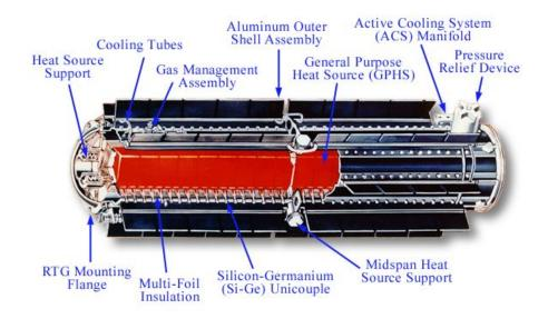
Figure 18. Radioisotope Thermoelectric Generator [From 56]
