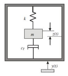
Figure 20. Model of Linear Inertial Generator [From 61]
