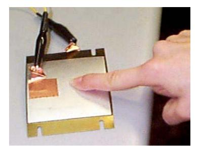
Figure 22. Piezoelectric Unimorph Heel Insert [From 65]
