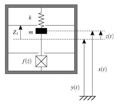
Figure 7. Model of Inertial Generator[From 26]
