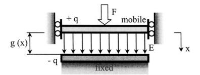
Figure 13. Attractive Force Generated by Electric Field [From 40]
