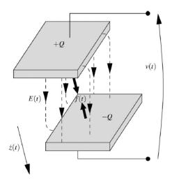
Figure 15. Electrostatic Transducer Constant Charge Operating Principle [From 41]
