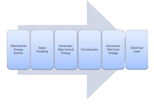
Figure 8. Energy Flow in MEMS Generator
