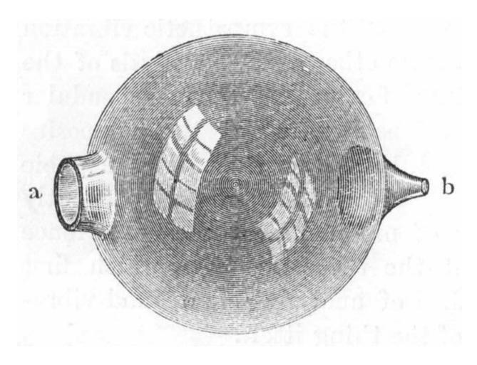
Figure 5. Schematic of Helmholtz Resonator [From 17]
