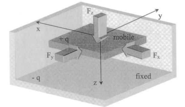
Figure 12. Potential Motion Directions of a Charged Mobile Plate when Attracted by Three Fixed Cartesian Wall-Plates [From 40]
