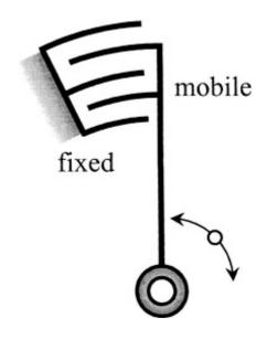
Figure 17. Rotary Electrostatic Transduction [From 40]
