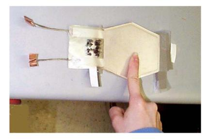
Figure 21. Piezoelectric Bimorph Stave for Insole [From 65]
