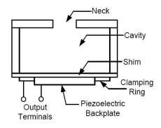
Figure 6. Electromechanical Helmholtz Resonator [From18]
