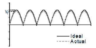
Figure 29. Voltage Output Rendered by Full Bridge Diode Rectifier [From 77]
