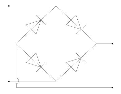
Figure 28. Full Bridge Diode Rectifier [From 77]
