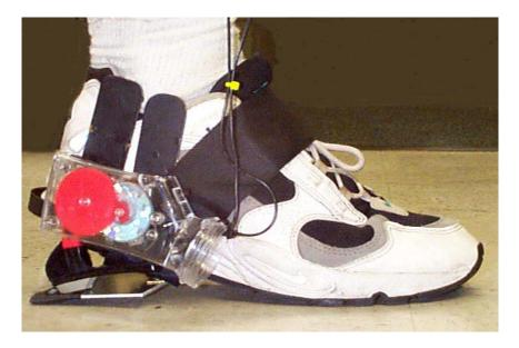
Figure 23. Rotary Electromagnetic Generator [From 65]
