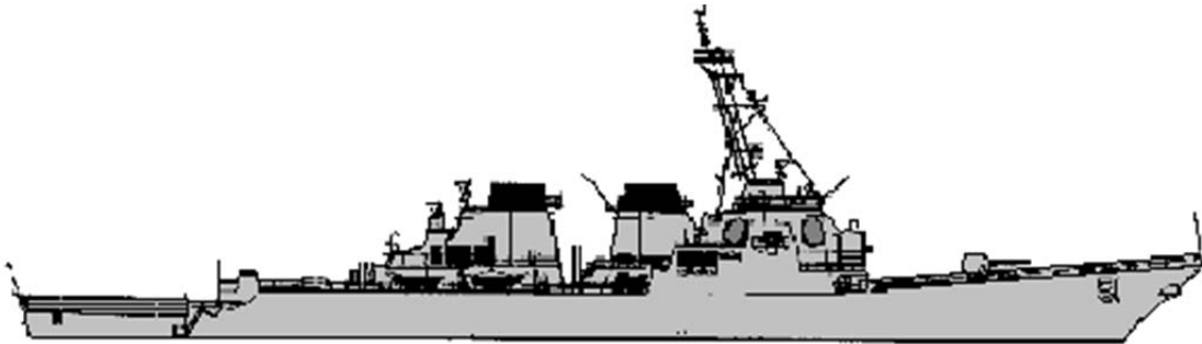
Figure 4. Arleigh Burke Guided Missile Destroyers (DDG 51–115) (FAS, 2014). The DDG has 12 installed modules. These destroyers are capable of carrying up to 96 missiles (from U.S. Navy Fact File, 2013).
