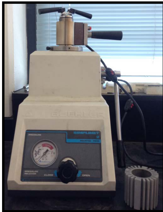
Figure 18. SimpliMet 2 mounting press used for hot mounting the samples in a phenolic puck.
