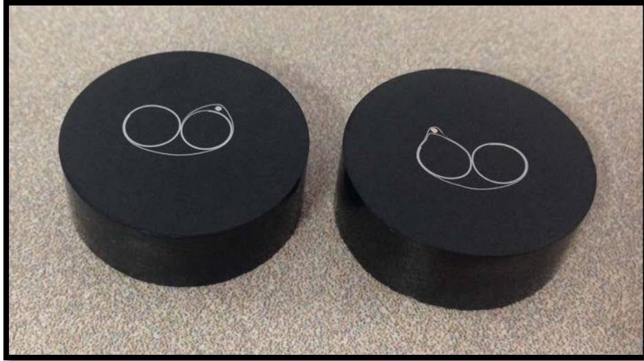
Figure 19. Phenolic pucks containing RES-treated substrates.
