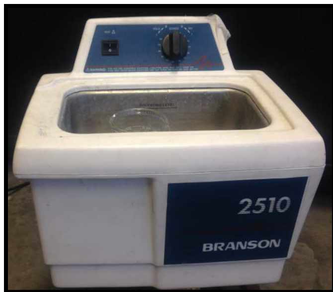
Figure 15. The substrates were placed in a glass beaker containing ethanol solvent then cleaned in a Branson 2510 Ultrasonic Cleaner.
