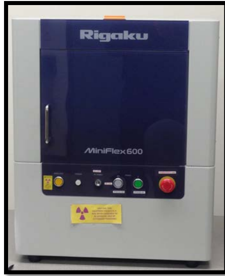
Figure 24. Rigaku MiniFlex 600 used for X-ray diffraction.
