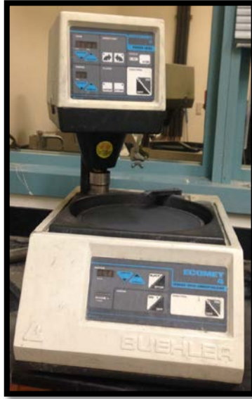
Figure 20. Buehler EcoMet 4 variable speed grinder-polisher with an AutoMet 2 power head.
