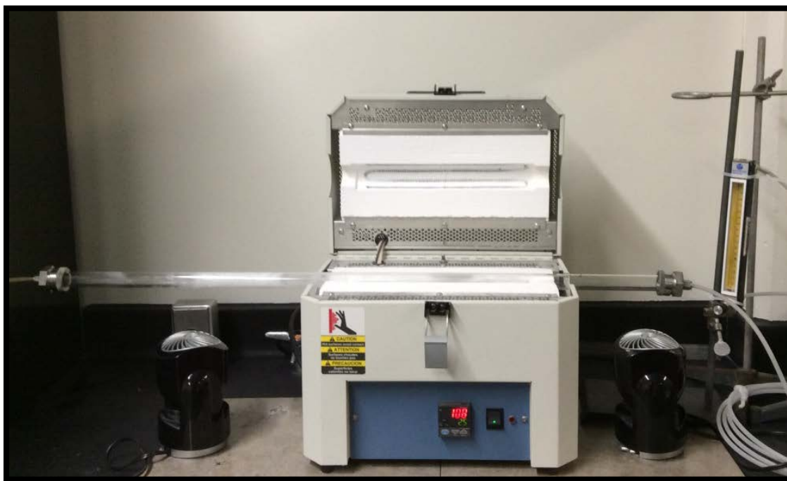
Figure 17. RES arrangement with quartz tube positioned in the clamshell Lindberg Blue M tube furnace and portable cooling fans.
