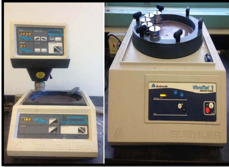
Figure 21. Buehler EcoMet 3 variable speed grinder-polisher with a AutoMet 2 power head (left) and a VibroMet 2 for final finishing (right).
