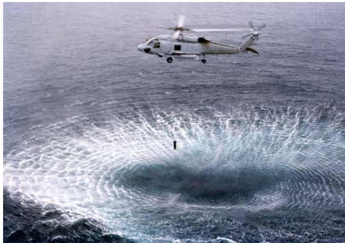
Figure 4. Aerial view of an SH-60F Seahawk helicopter lowering a dipping sonar into the Pacific Ocean (image from Wikimedia Commons http://commons.wikimedia.org ).
