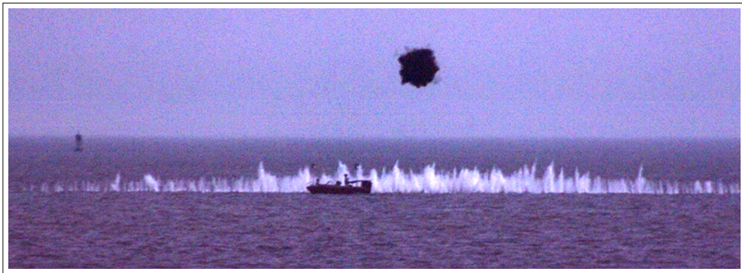
Figure 2.4: An air burst of a 57mm Bofors MK III projectile above its intended target.
