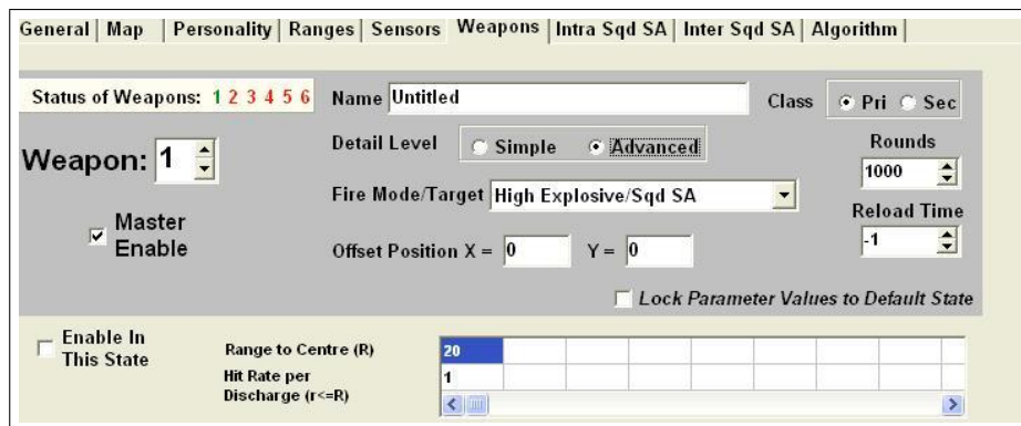
Figure 2.9: MANA setup panel for a high explosive weapon.
