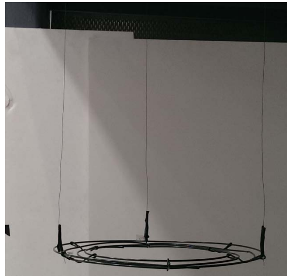
Figure 14 Trifilar Pendulum Setup.
