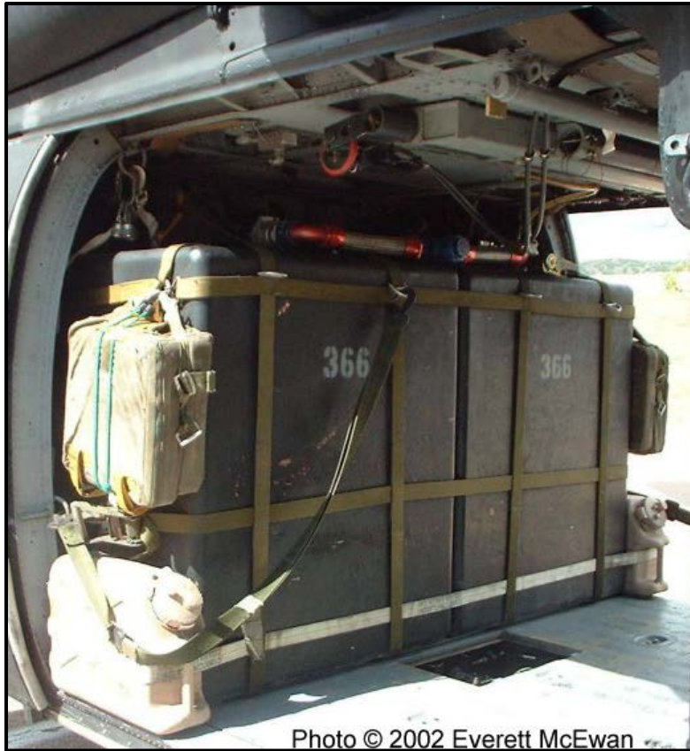
Figure 1. Fuel cell on MH-60 Blackhawk helicopter[3]
