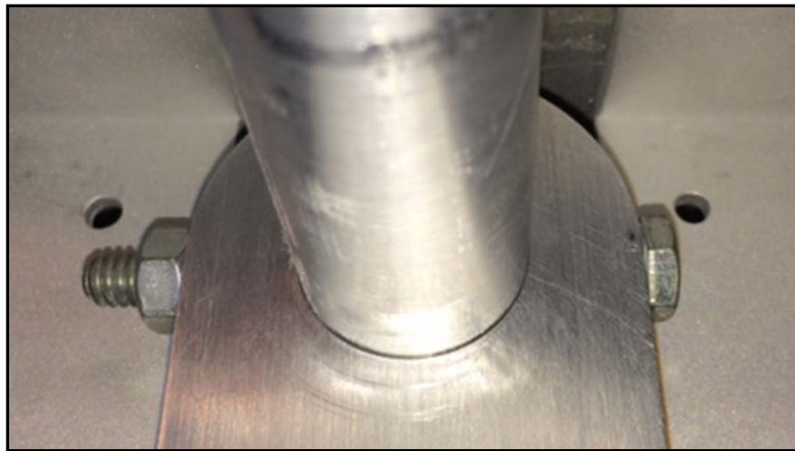
Figure 18. Attachment point for rotating rod and pendulum arm
