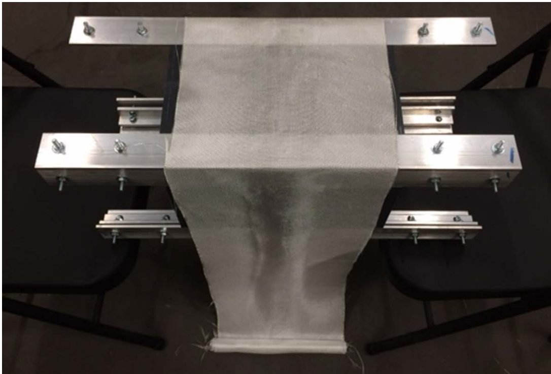
Figure 6. First layer of E-glass laid on form during fabrication
