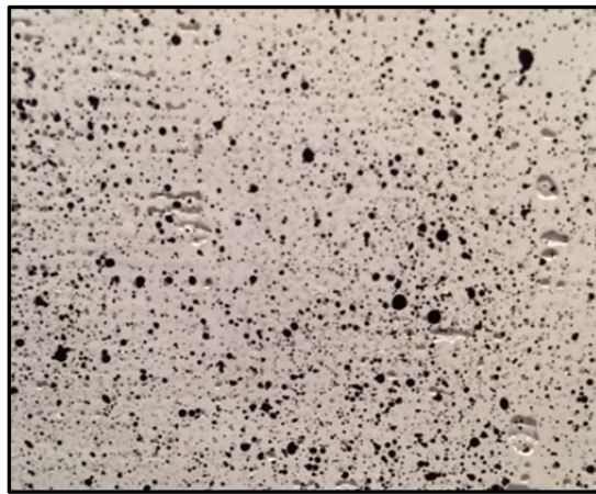
Figure 22. Speckle Pattern for Digital Image Correlation.
