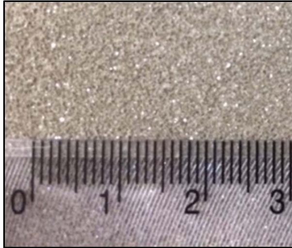
Figure 23. Close Cell Vinyl Foam for Baffles.
