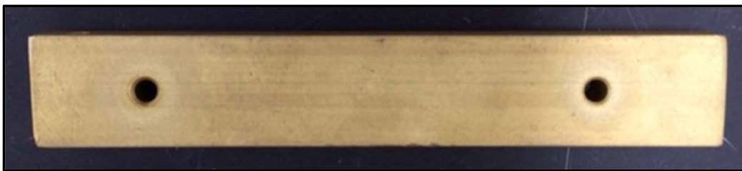
Figure 36. Brass Weight Attached to Pendulum Arm.
