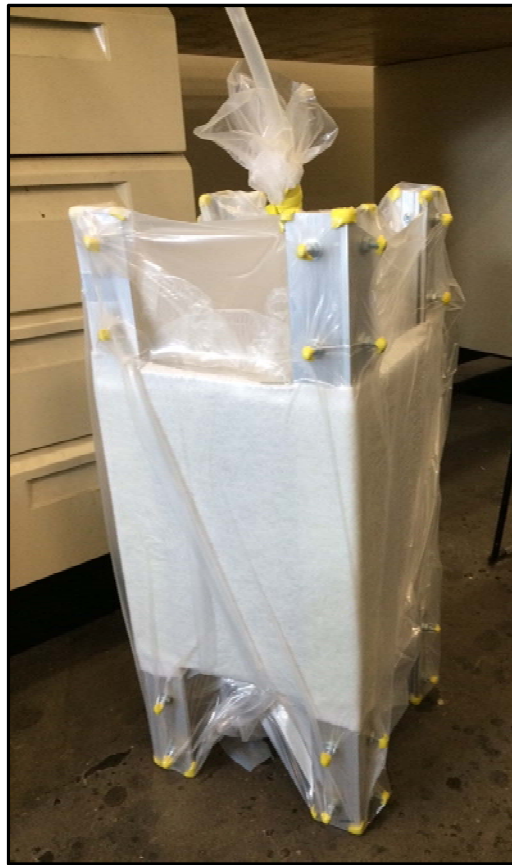
Figure 16. Form and Composite Under Vacuum After Layup.
