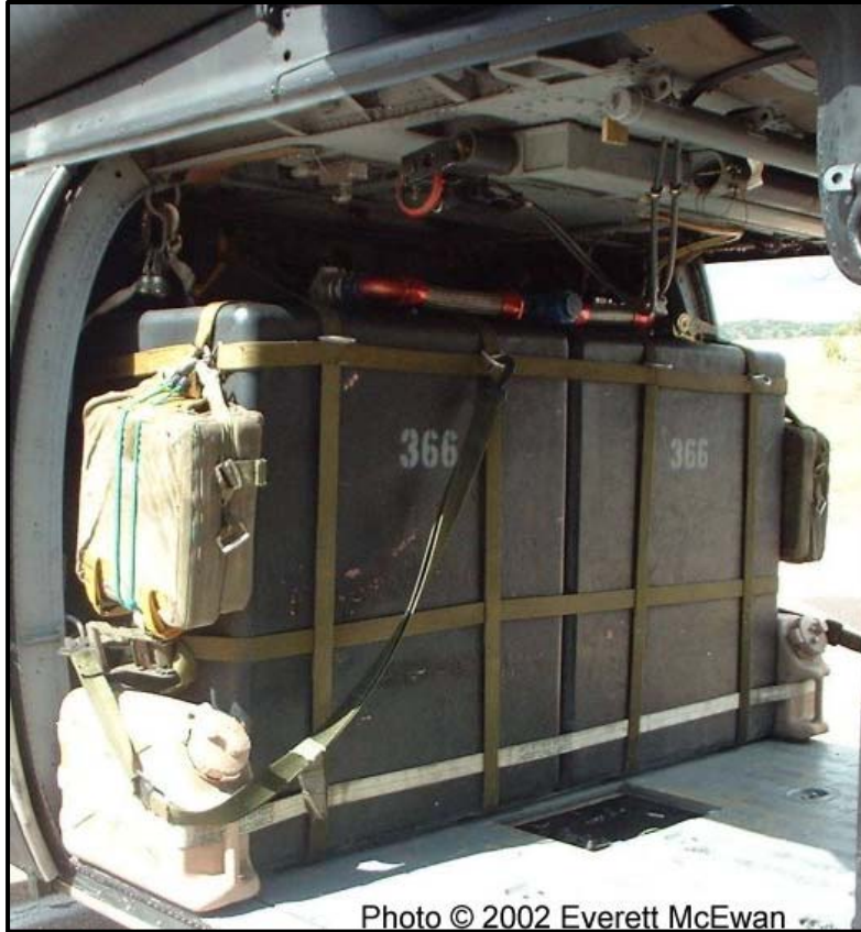
Figure 1. Fuel Cell on MH-60 Blackhawk Helicopter. Source: [3].
