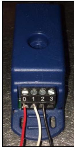
Figure 78. Strain Gage Wire Leads into NI-9945 Screw Terminal Adaptor.
