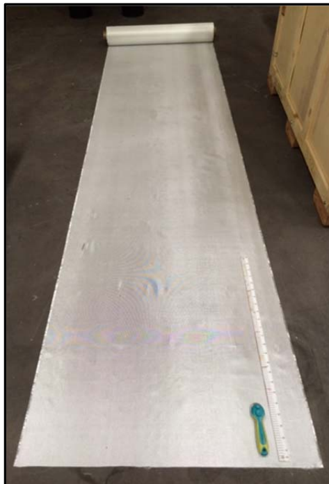
Figure 13. Roll of E-Glass Ready to be Cut into Layers for Composite Fabrication.
