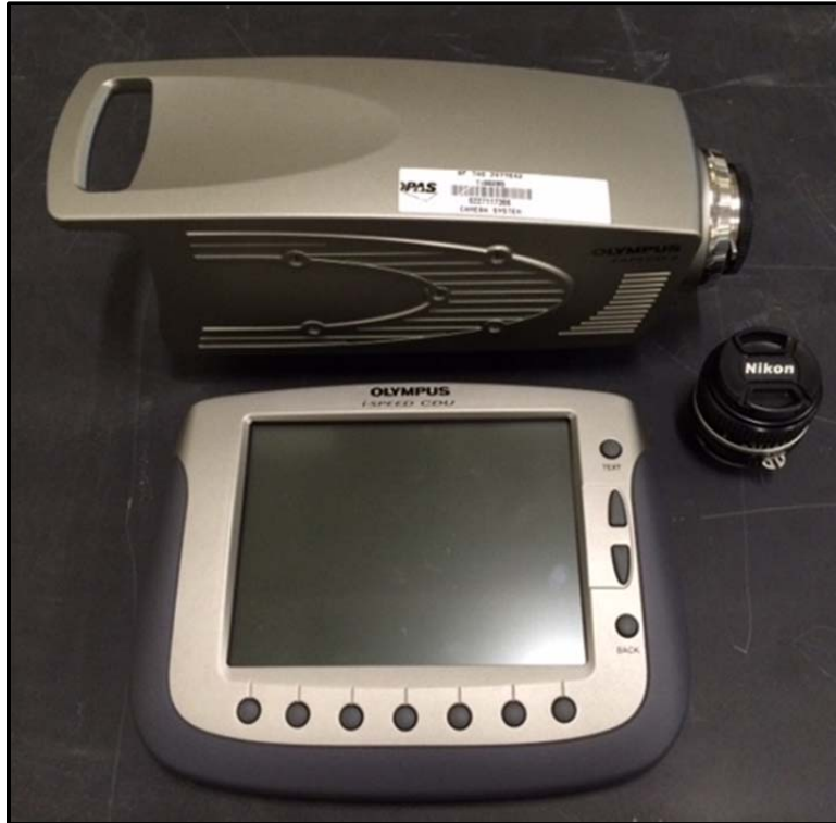
Figure 43. Olympus® High-Speed Camera, Screen, and Nikon® Lens.
