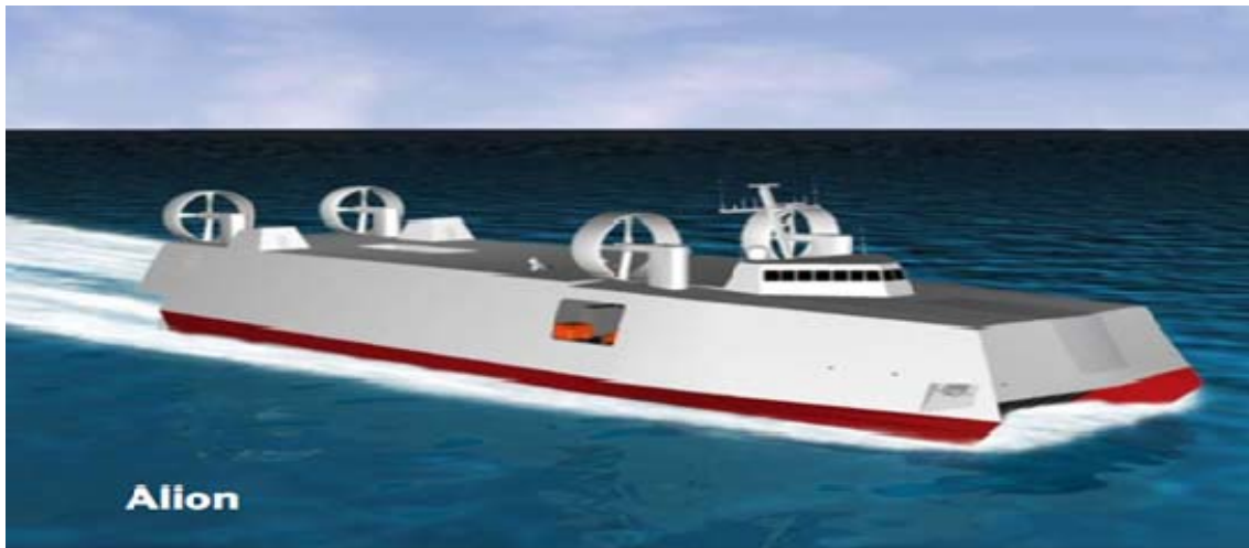
Figure 5. The Alion Transformable Craft prototype is built on a catamaran-type frame. (From Chang, 2008)
