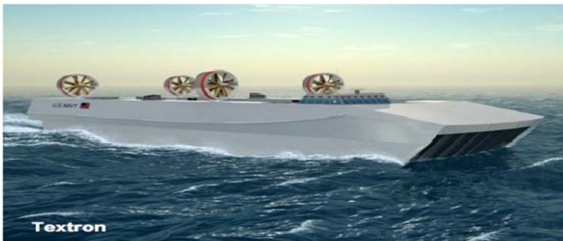
Figure 6. The Textron Transformable Craft prototype closely resembles the LCAC, which Textron also designed; both have an open cargo area. (From Chang, 2008)
