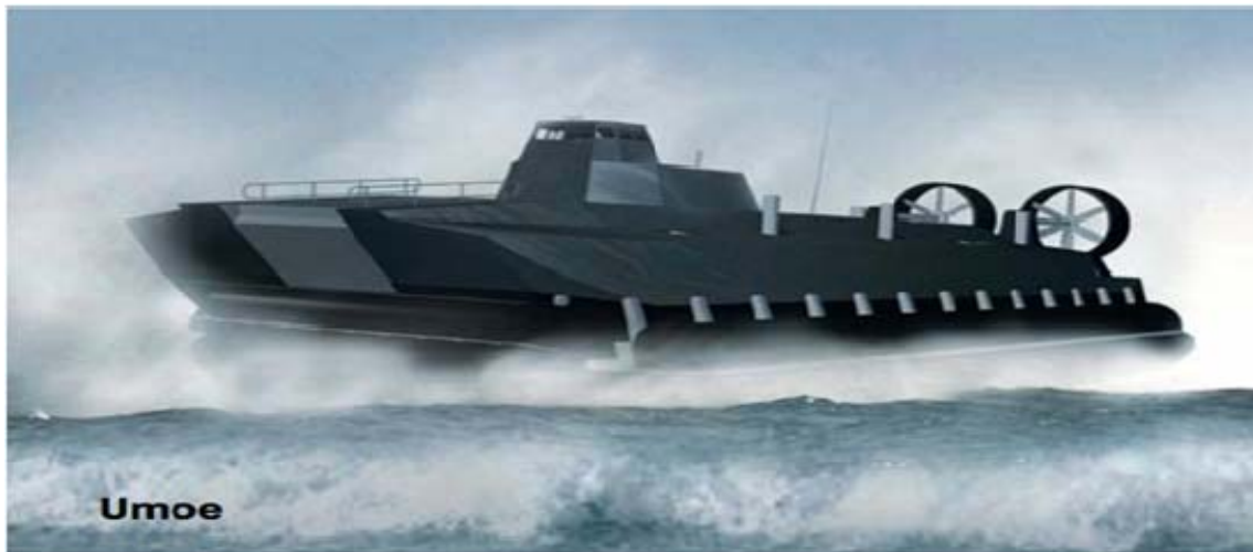
Figure 7. The Umoe Transformable Craft prototype has a high-speed surface effect hull design with closed cargo area. (From Chang, 2008)
