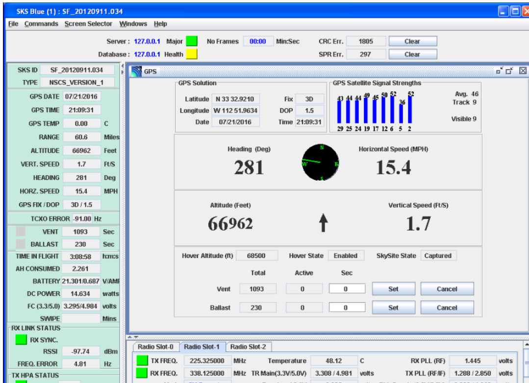
Figure 8. Image of Flight Control Software Utilized for SkySat Operations.
