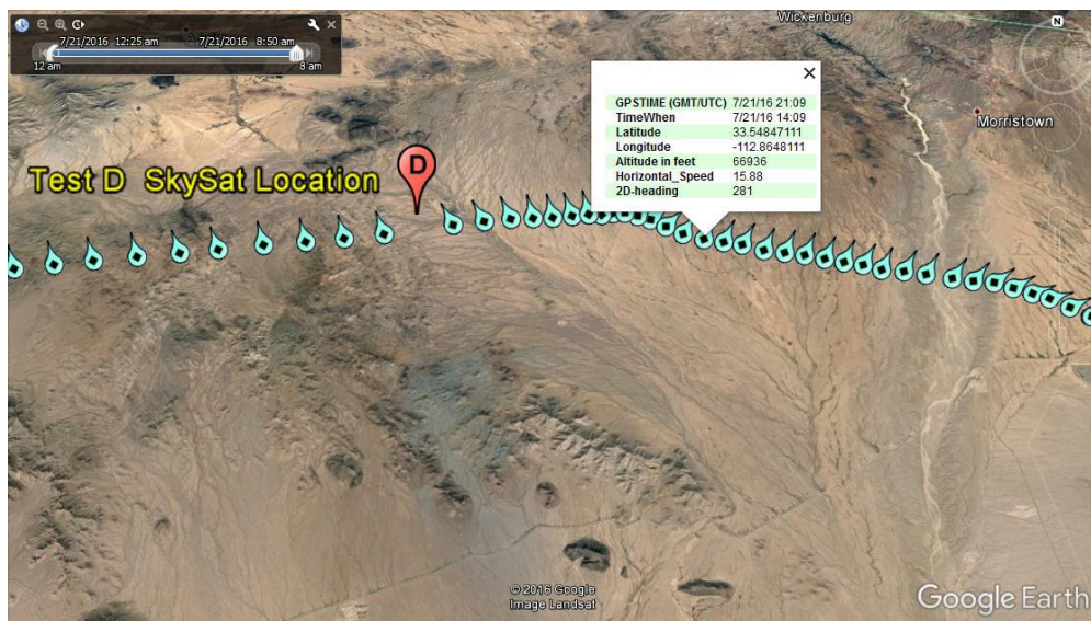
Figure 5. Sample of Data Captured by SkySat Telemetry.
