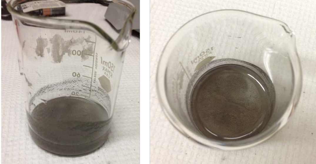
Figure 13. Nickel Powder wetted with H_2O_2
