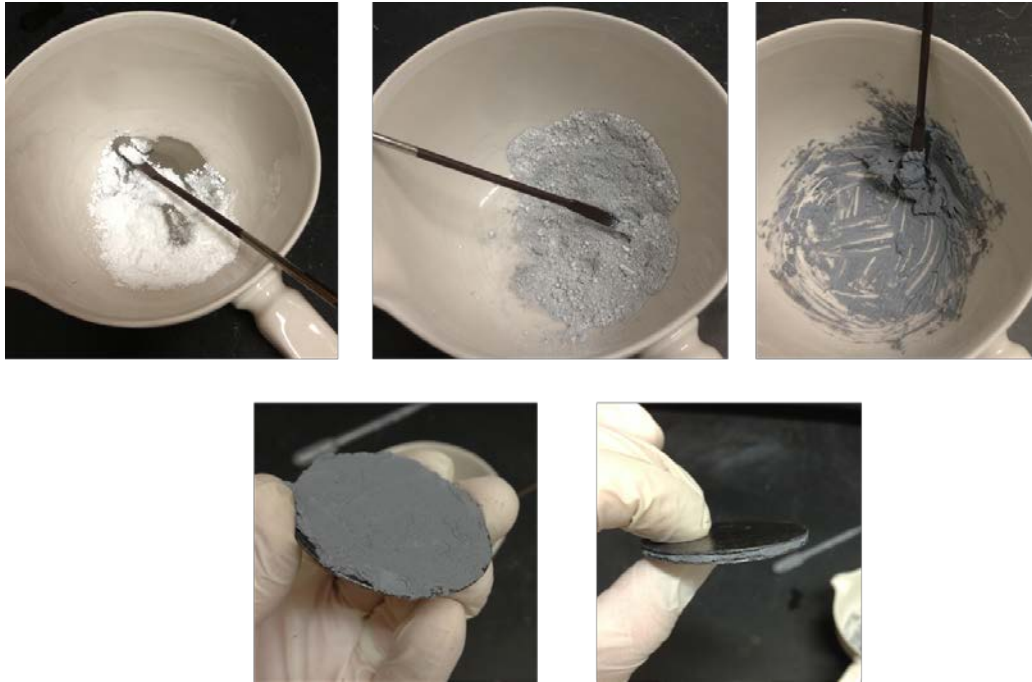
Figure 16. Composite Dielectric Capacitor Preparation Process
