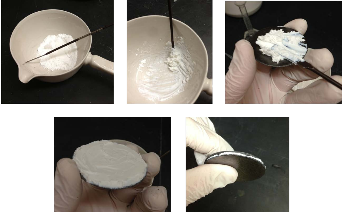
Figure 12. HSA Electrolyte Capacitor Preparation Process
