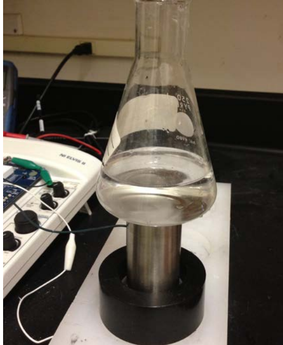
Figure 11. Capacitor Test Jig Weight Arrangement
