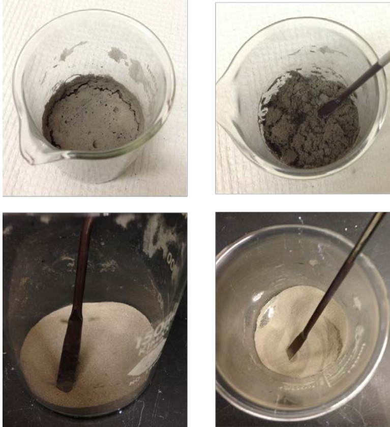
Figure 14. Nickel Powder Surface Treatment Drying Process
