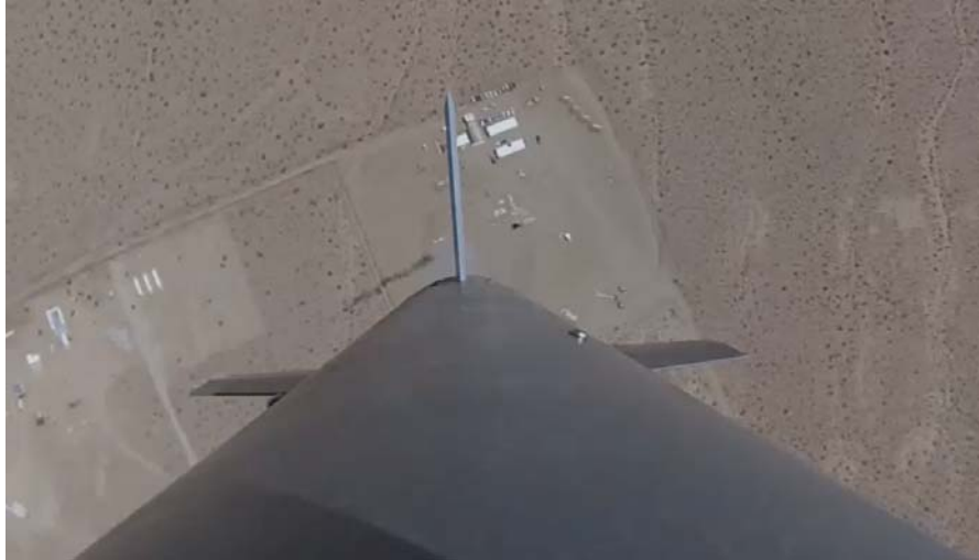
Figure 38. Pre-actuated Fins ( 0^\circ Deflection)
