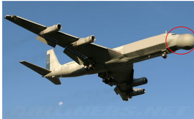
Figure 10. A few examples of conformal arrays. (a) Conformal array on sonar seekers. Image from [26], and (b) Image of the EL/M-2075 Phalcon solid-state L-band conformal mounted array radar system on an aircraft. Image extracted from [27]. The images shown are for illustrative purposes.
