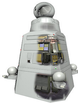
Figure 1. Thales I-MAST integrated mast with sensor systems accommodated on and within the mast structure. Image from [3] shown for illustrative purposes.
