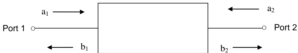
Figure 28 Two-port, two-pin component schematic with signal wave directions. Image extracted from ADS Systems’ RF system Budget Analysis [52]. a_1 denotes the signal wave into port 1, b_1 denotes the wave out of port 1, a_2 denotes the signal wave into port 2 and b_2 denotes the signal wave out of port 2.
