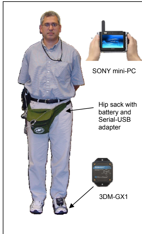
Figure 16. User with IMMU attached to foot and SONY mini-computer.
