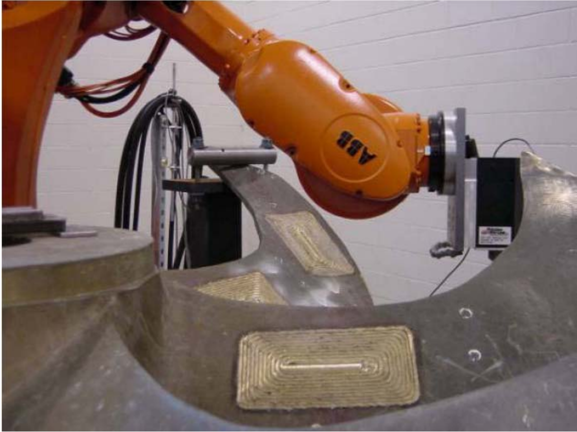
Figure 5. Area Processing of a Marine Propeller (From [13])
