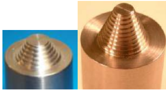
Figure 12. 6mm and 13mm FSP tools (From [13])
