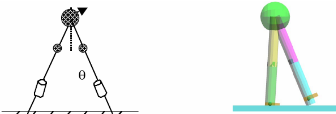
Figure 28: Compass-like biped model, after (Miyakoshi et al., 2001)
