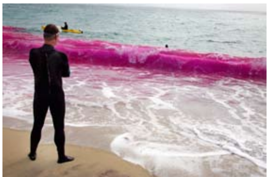
MacMahan releases dye in surf zone to measure dispersion, material transport.
