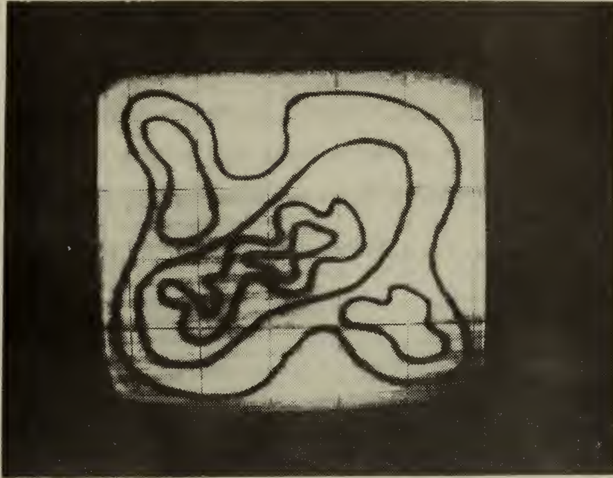
FIGURE 3. HP-1300A DISPLAY OF SCANNED CONTOURS TRANSPARENCY
