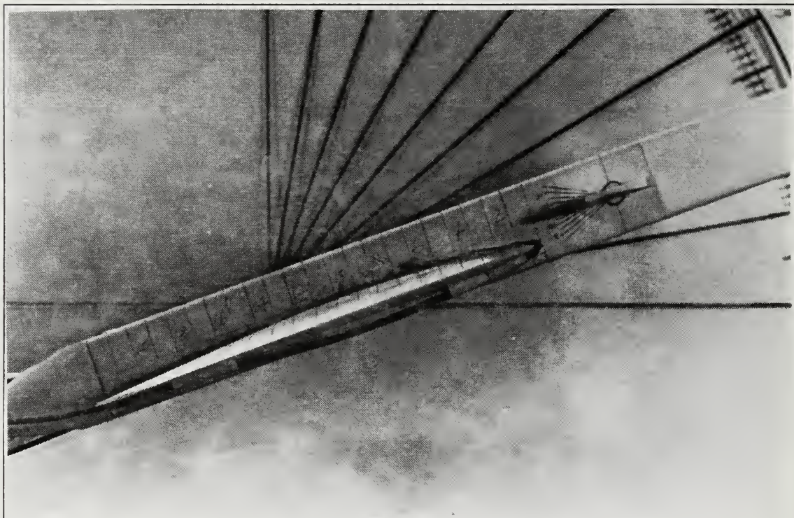
Figure 63. Wing Root Vortex Flow, \alpha=20^\circ , K=-0.16 , \delta=0^\circ , K_c=0
