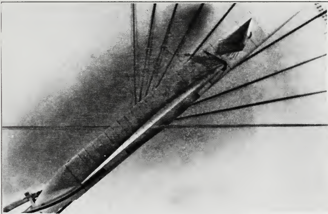
Figure 32. Wing Root Vortex Flow, Static Case, \alpha=40^\circ , \delta=+25^\circ
