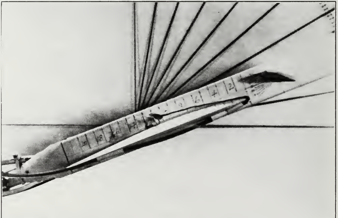
Figure 41. Wing Root Vortex Flow, Static Case, \alpha=20^{\circ} , \delta=-25^{\circ}
