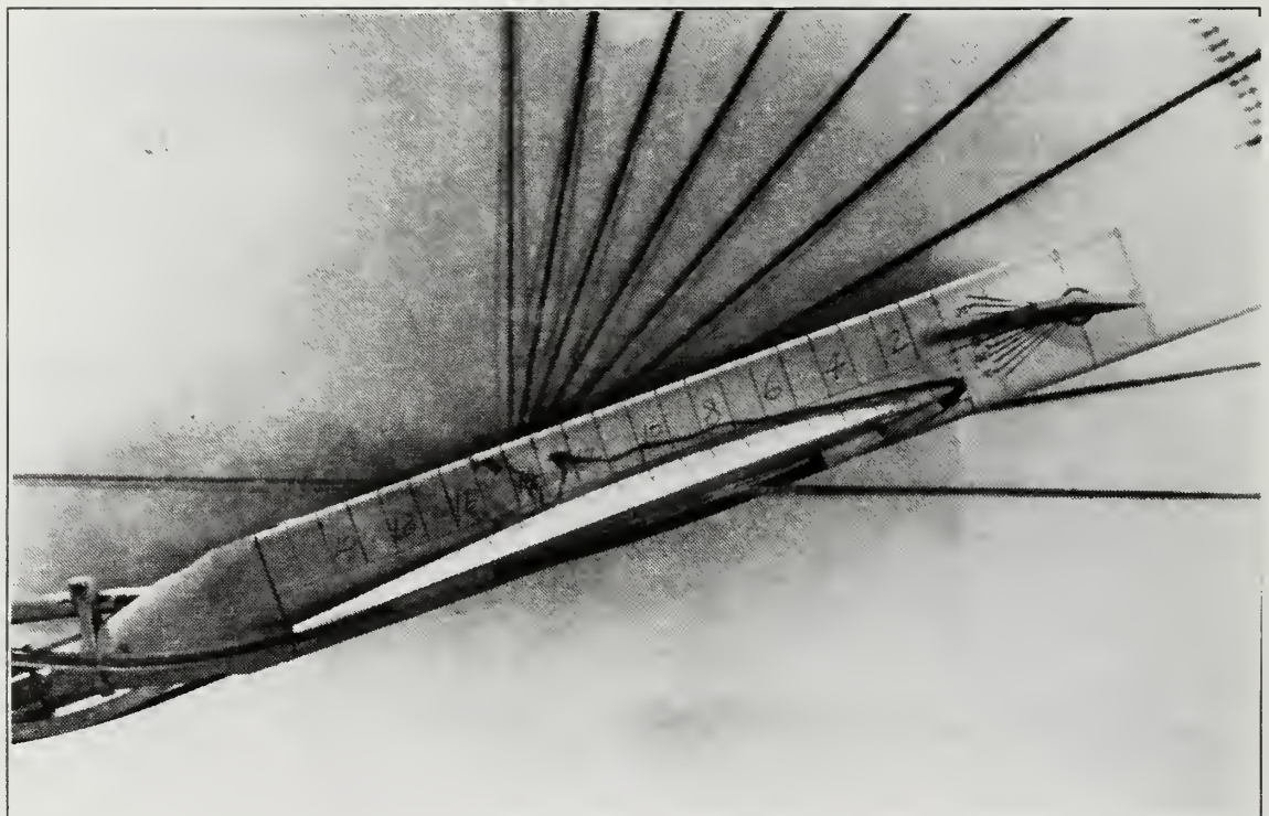
Figure 35. Wing Root Vortex Flow, Static Case, \alpha=20^\circ , \delta=-10^\circ
