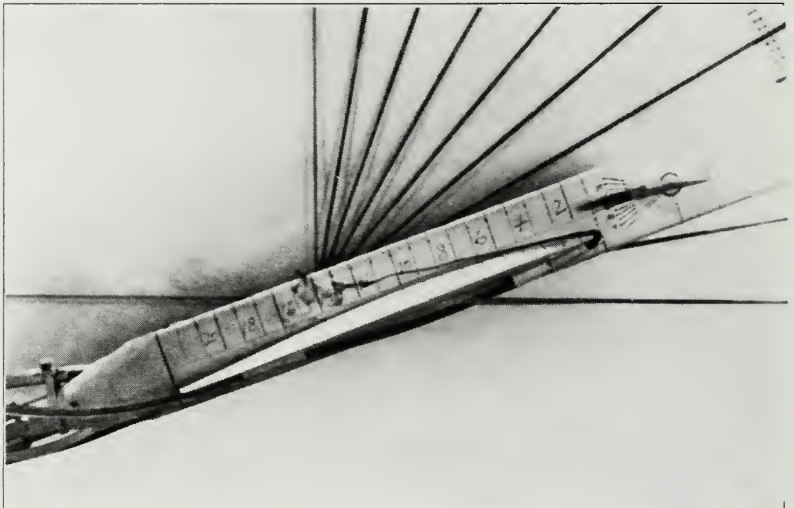
Figure 33. Wing Root Vortex Flow, Static Case, \alpha=20^\circ , \delta=-5^\circ
