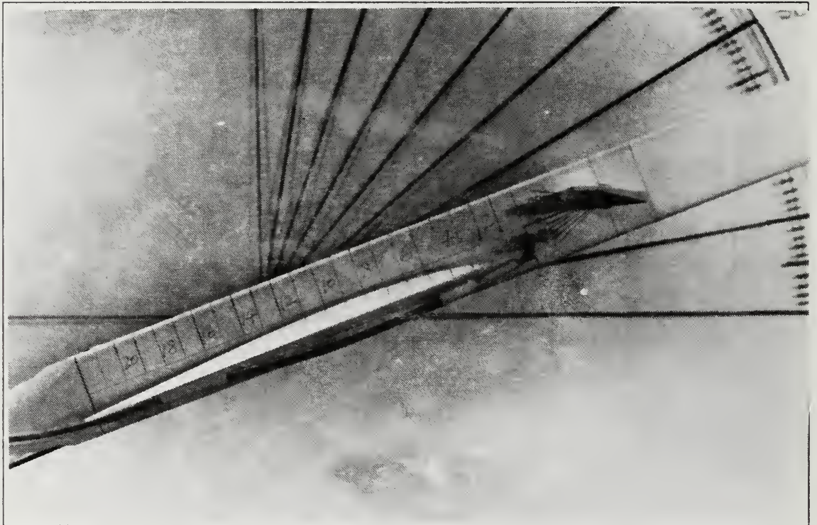
Figure 51. Wing Root Vortex Flow, \alpha=20^\circ , K=0 , \delta_a=\pm 25^\circ , K_c=10.4
