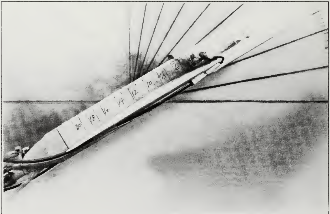
Figure 71. Wing Root Vortex Flow, \alpha=30^\circ , K=-0.16 , \delta_a=+/-5^\circ , K_c=1.7
