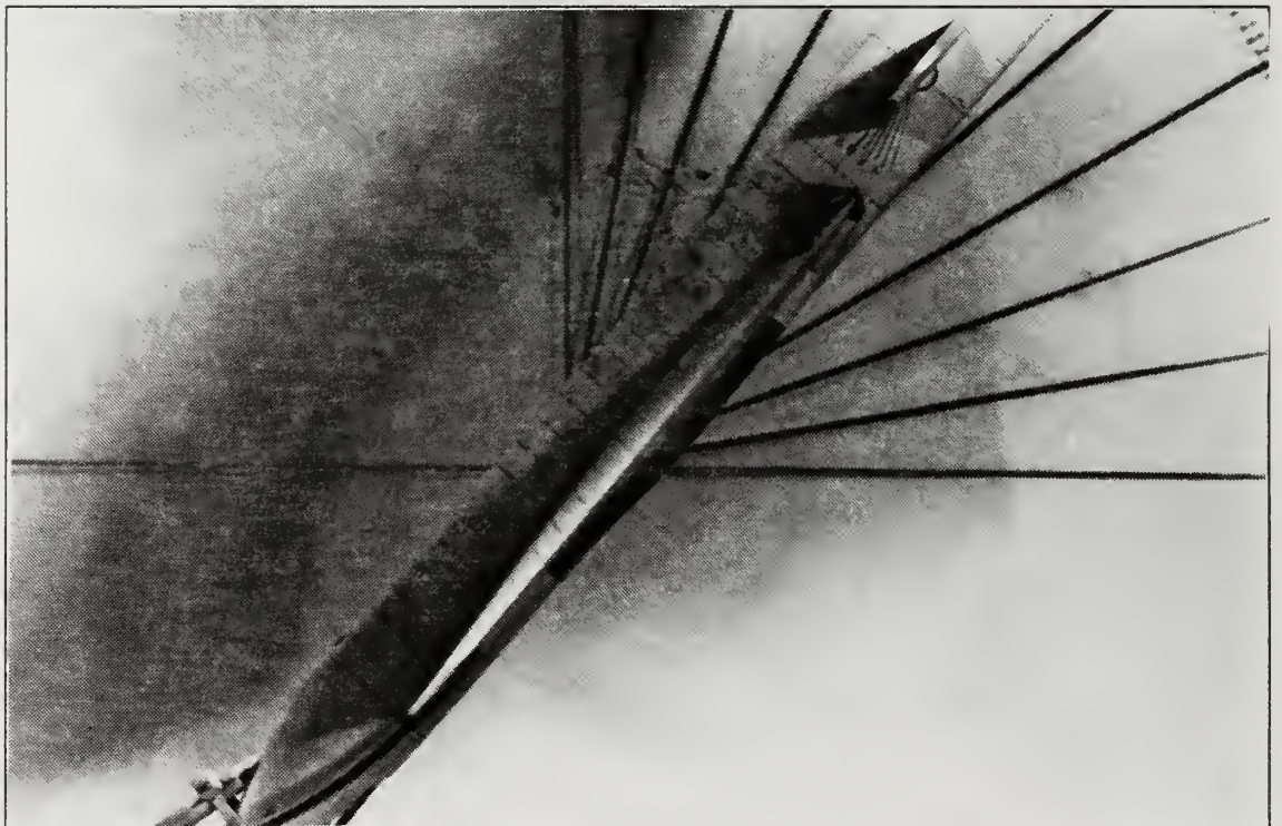
Figure 17. Wing Root Vortex Flow, Static Case, \alpha=50^\circ , \delta=0^\circ
