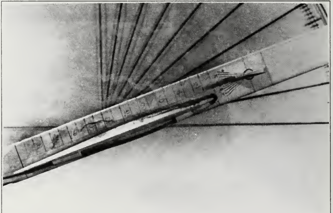
Figure 43. Wing Root Vortex Flow, \alpha=20^\circ , K=0 , \delta_a=\pm 5^\circ , K_c=1.7
