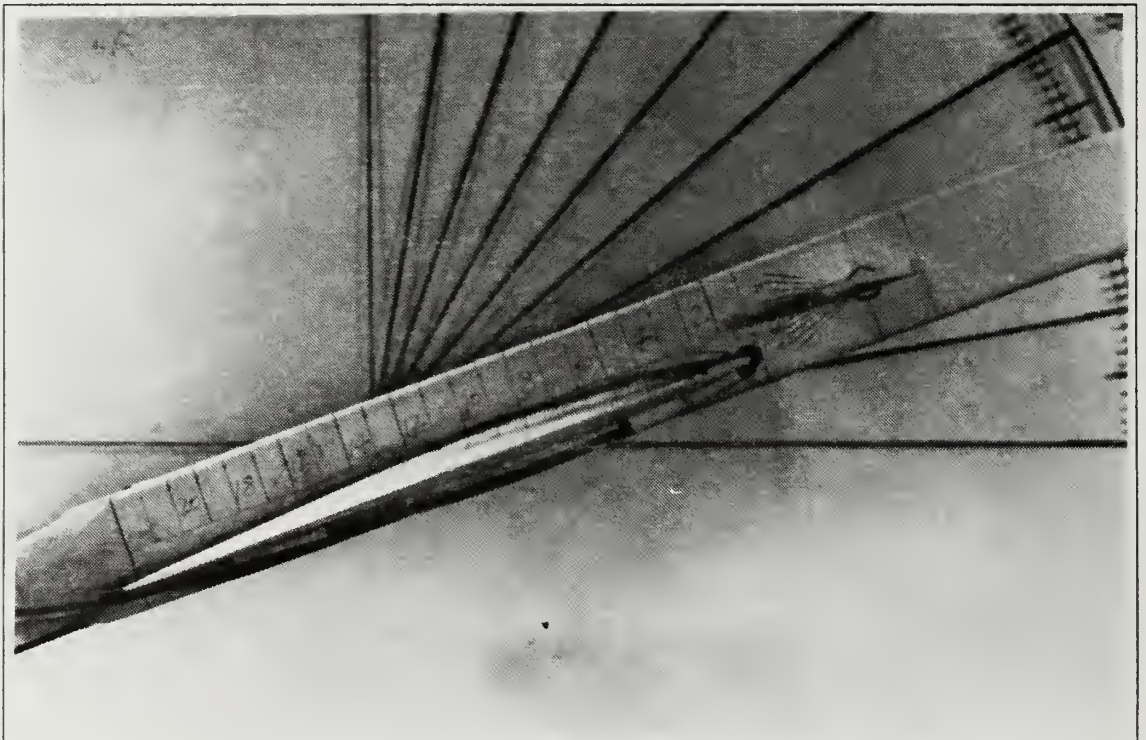
Figure 53. Wing Root Vortex Flow, \alpha=20^\circ , K=0.08 , \delta=0^\circ , K_c=0
