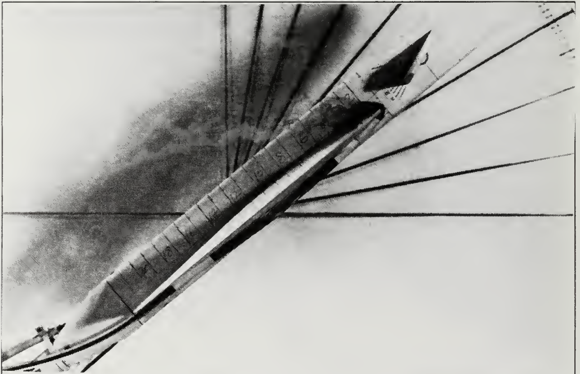
Figure 29. Wing Root Vortex Flow, Static Case, \alpha=40^\circ , \delta=+20^\circ
