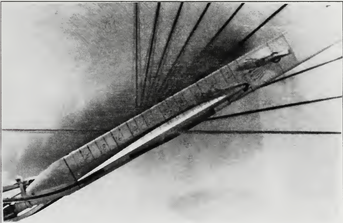
Figure 34. Wing Root Vortex Flow, Static Case, \alpha=30^\circ , \delta=-5^\circ
