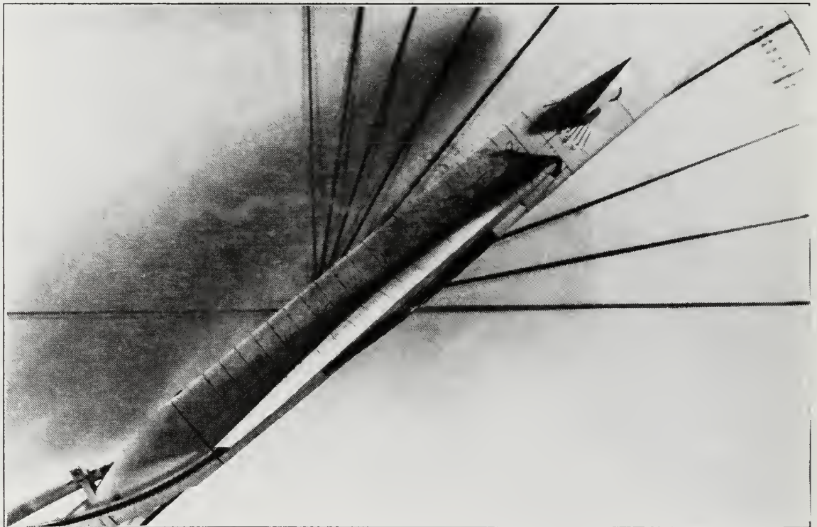
Figure 23. Wing Root Vortex Flow, Static Case, \alpha=40^\circ , \delta=+10^\circ
