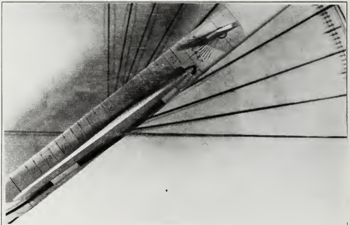
Figure 45. Wing Root Vortex Flow, \alpha=40^\circ , K=0 , \delta_a=\pm 5^\circ , K_c=1.7
