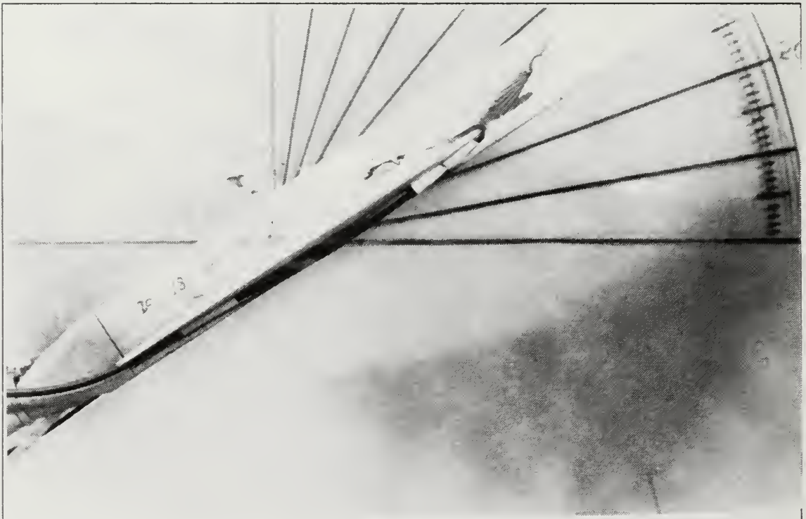
Figure 79. Wing Root Vortex Flow, \alpha=30^\circ , K=0.16 , \delta_a=\pm 25^\circ , K_c=1.7
