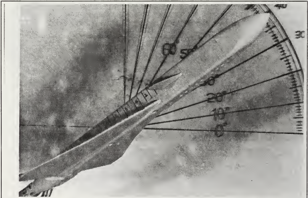
Figure 35. Wing Root Vortex Flow, Positive Sideslipping ( k=0.08 ), \alpha=35^\circ , \beta=20^\circ
