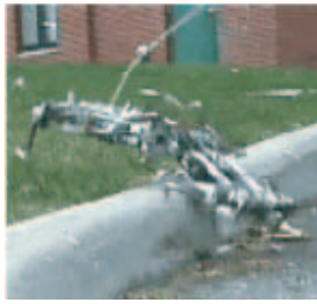
Fig. 2. Whegs TM II flexing its body as it climbs over a curb
