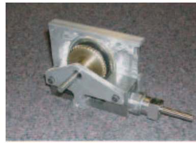
Fig. 11. Whegs TM III body joint drive shaft (right) and middle axle (left) in coaxial arrangement
