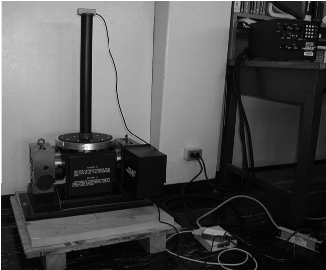
Fig. 8. Experimental setup using a HAAS precision tilt table.
