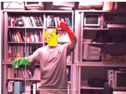
Figure 1. Head and hand detection using depth from stereo, illumination-specific color segmentation, and knowledge of typical body characteristics. 17
