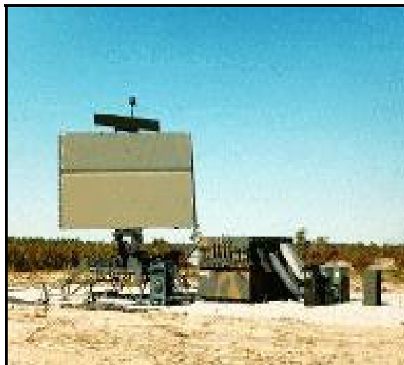
Figure 5. AN/TPS-75 Ground Theater Air Control System Radar System
