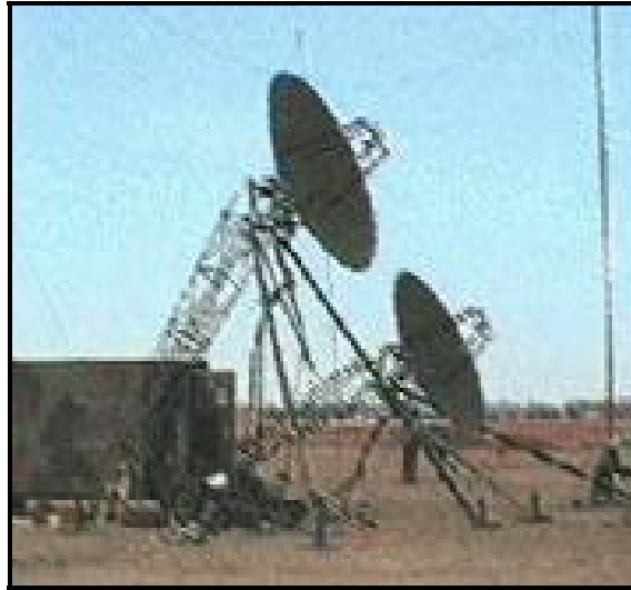
Figure 4. AN/TRC-170 Tropospheric Scatter Microwave Radio Terminal
