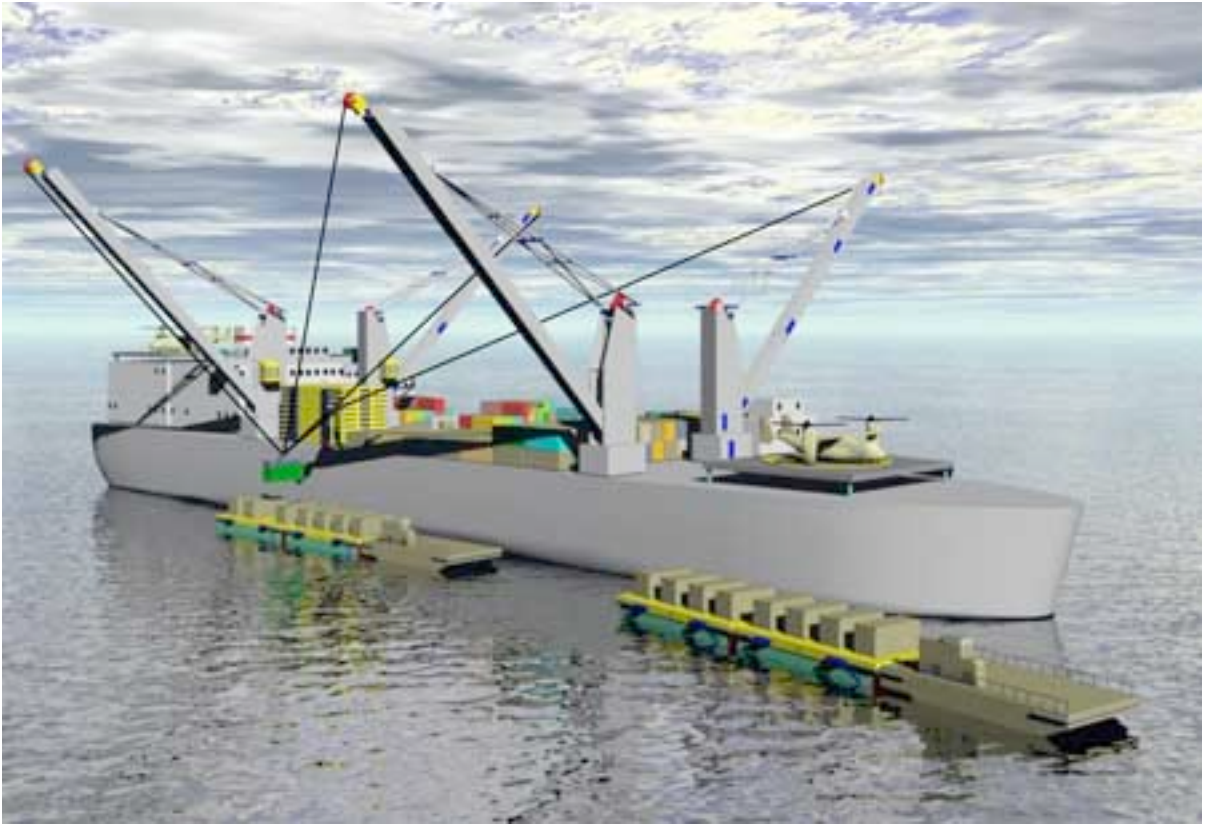
Figure 21. Illustration of use of AUTOLOG for discharging cargo to lightering [10].
