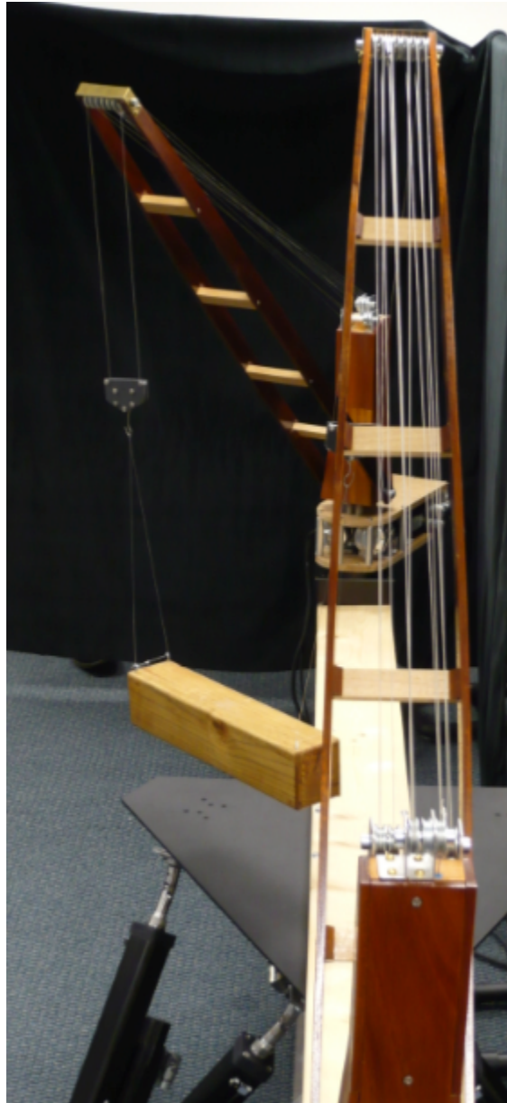
Figure 30. End view of model of the dual crane system with jibs at arbitrary slew angles. The jibs clearly do not lie in a common plane. The vertical offset of the hoist falls is still discernable.
