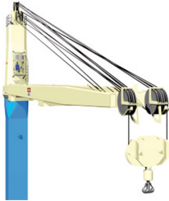
Figure 15. Typical wire-luffing jib crane on a single pedestal foundation.
