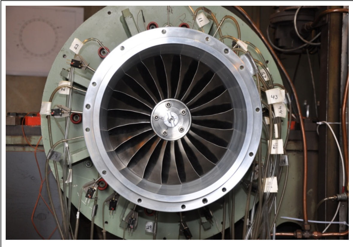
Figure 2. Transonic Compressor Rig with Forward Swept Fan
