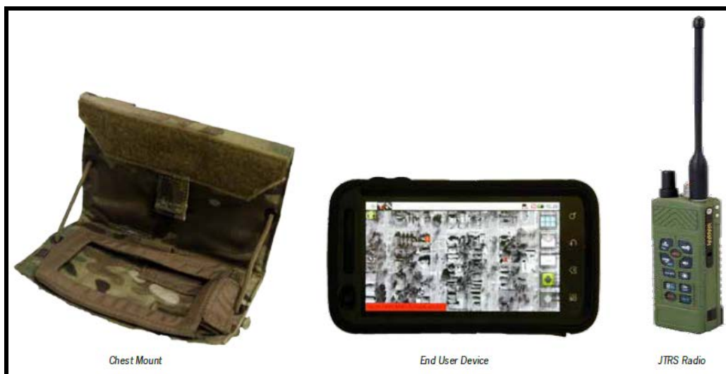
Figure 26. NW End User Device (EUD) With JTRS Radio. (From PEO–Soldier, 2011)
