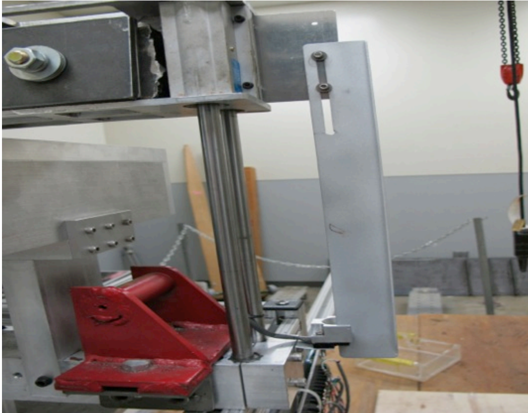
Figure 3. Trigger mechanism and sensor.
