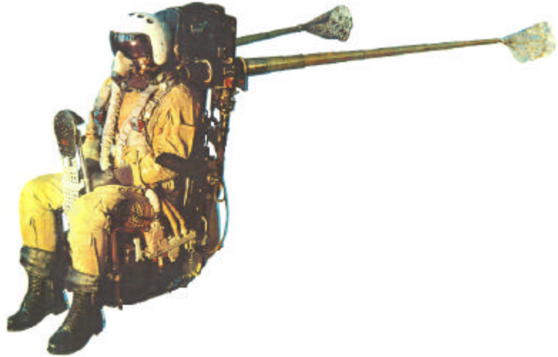
Figure 9.9 K-36D Ejection Seat
