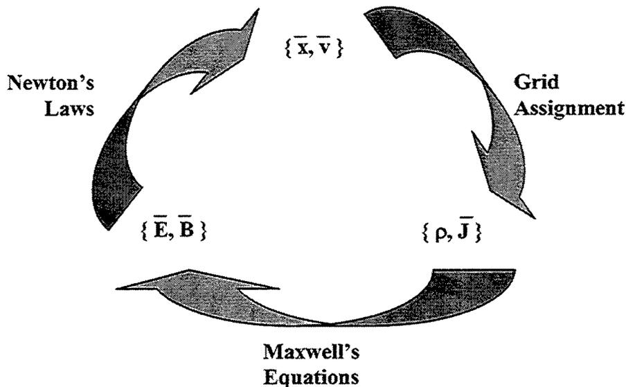
Figure 3. Particle Simulation Cycle. Note:  $\bar{x}$  is position,  $\bar{v}$  is velocity,  $\rho$  is charge density,  $\bar{J}$  is current,  $\bar{E}$  is the electric field, and  $\bar{B}$  is the magnetic field.
