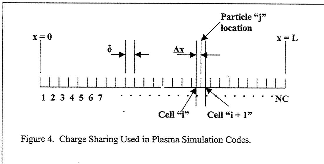
Figure 4. Charge Sharing Used in Plasma Simulation Codes.
