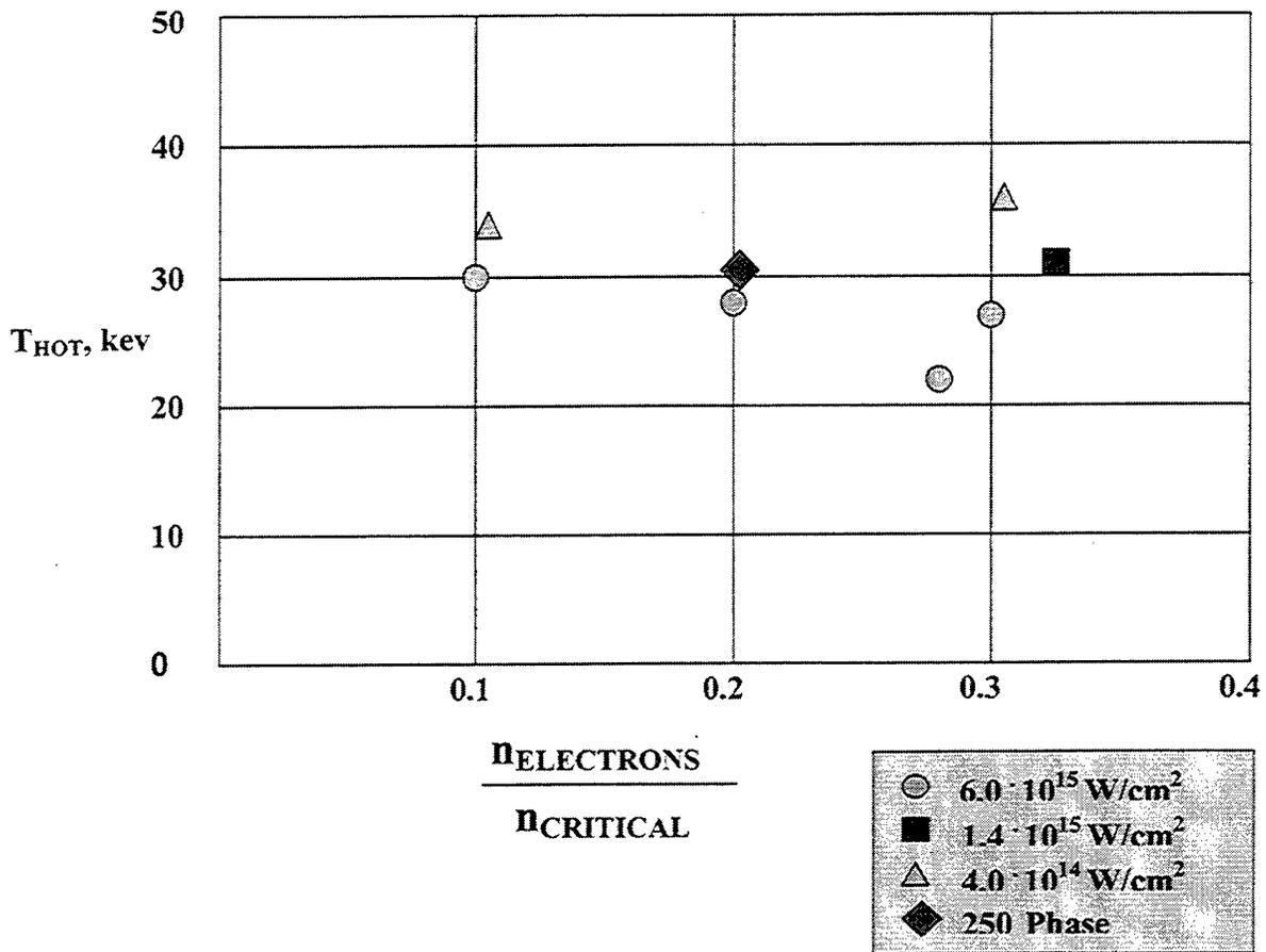
Figure 18. Measured Experimental Values for  $T_{HOT}$  Electrons [Reference 5].
