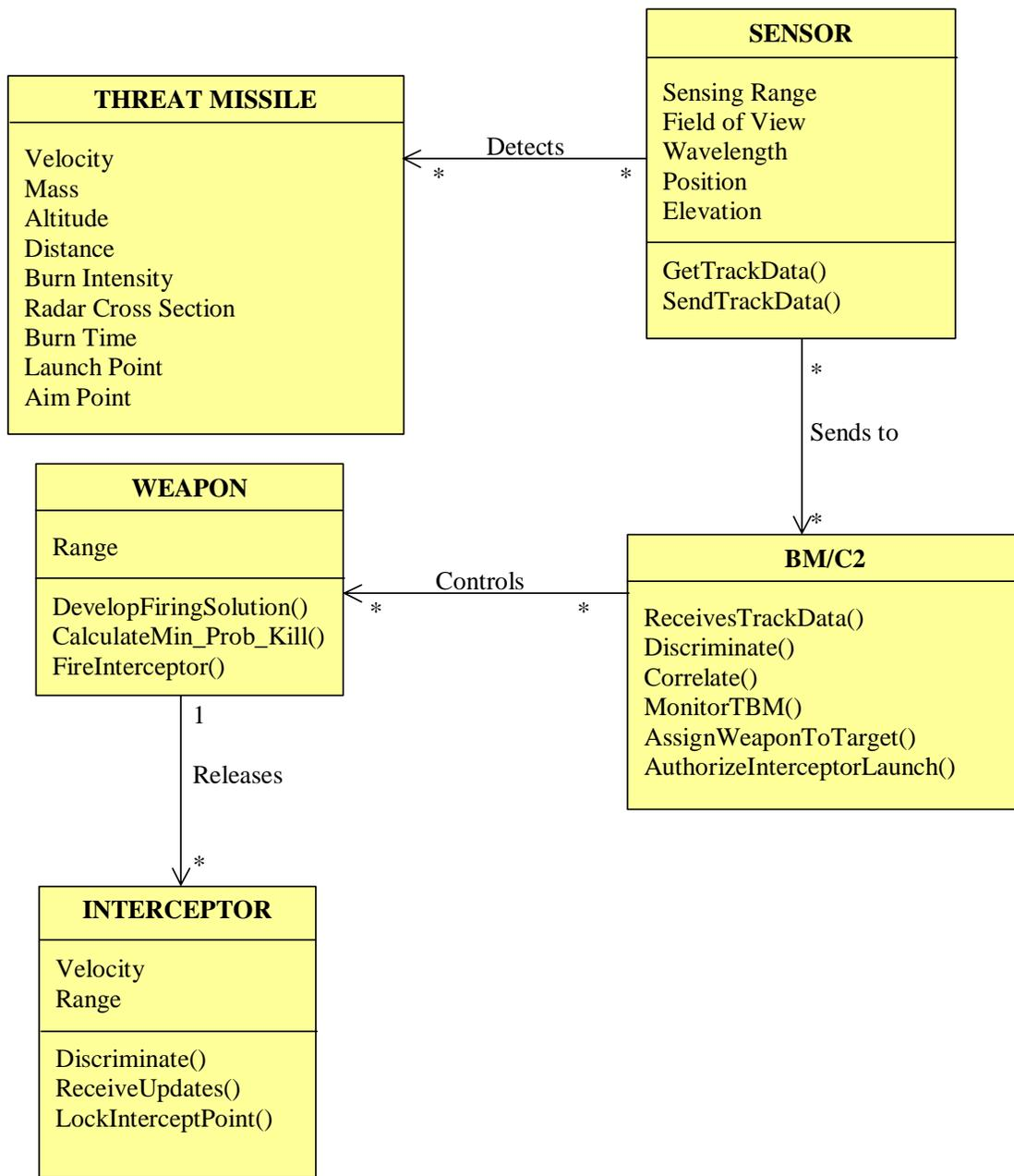
Figure 3. Class Diagram of Hypothetical Missile Defense System-of-Systems
