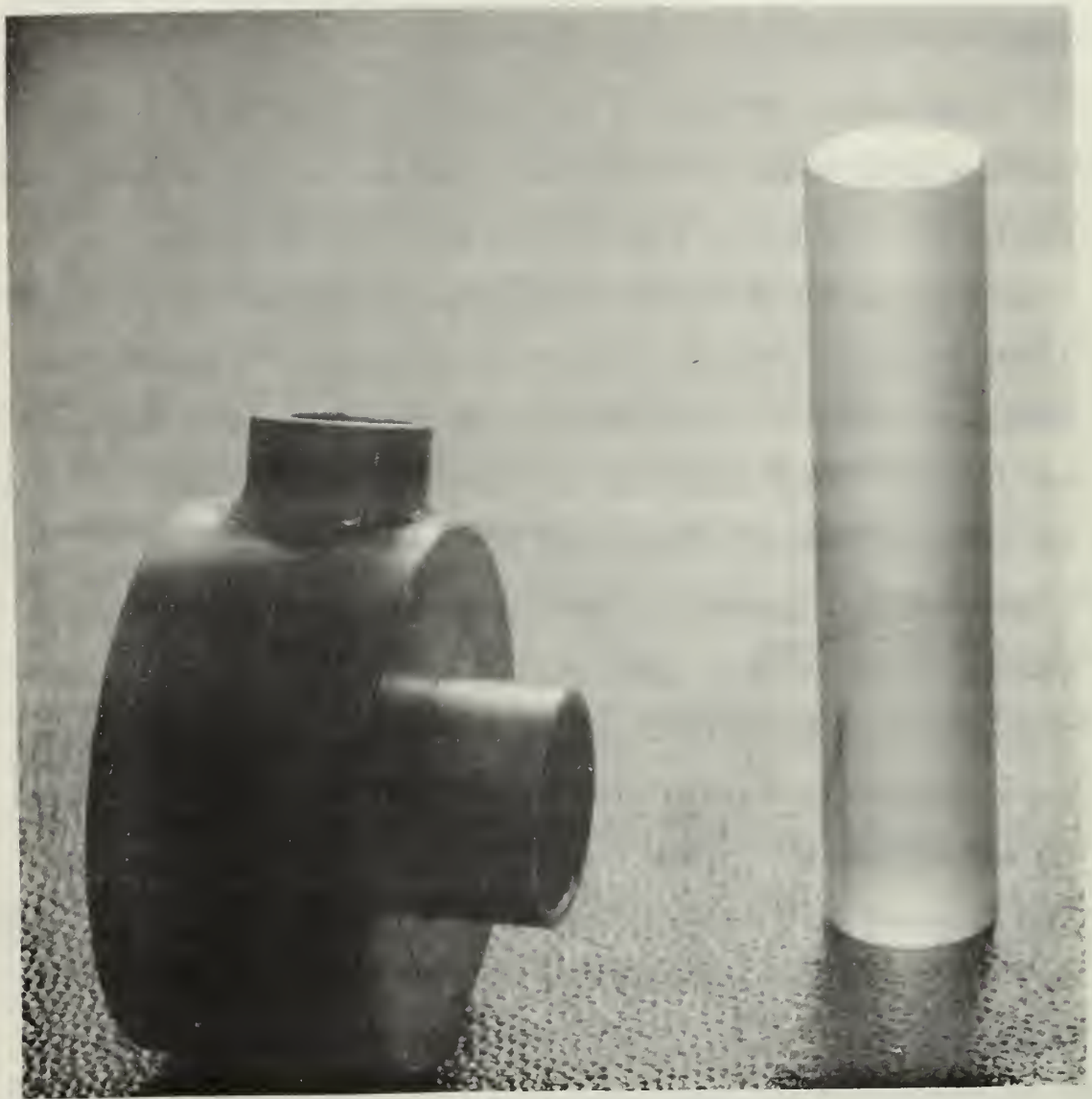
Figure 4-1. Ruby sample with bonded transducer on upper end and reentrant cavity. Microwave coupling loop screws into top of cavity.
