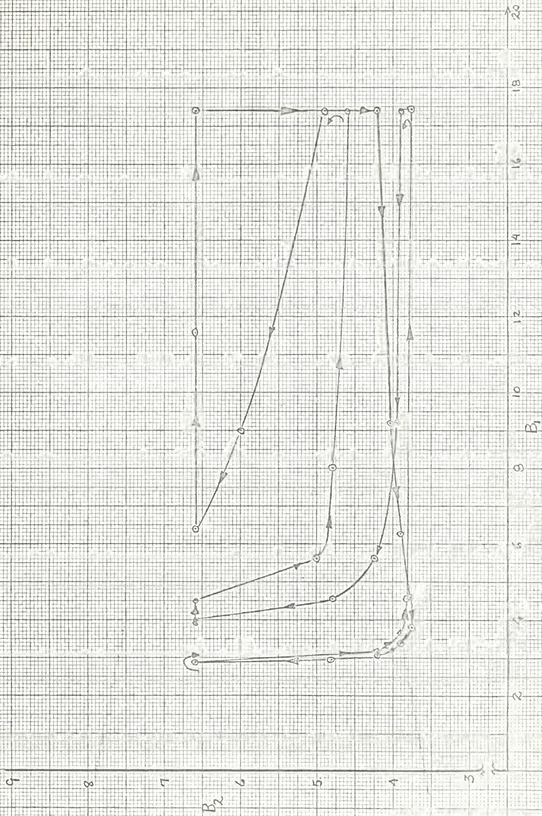
Figure IV-9. B_1 - B_2 plane trajectory for 30 volt step input.
