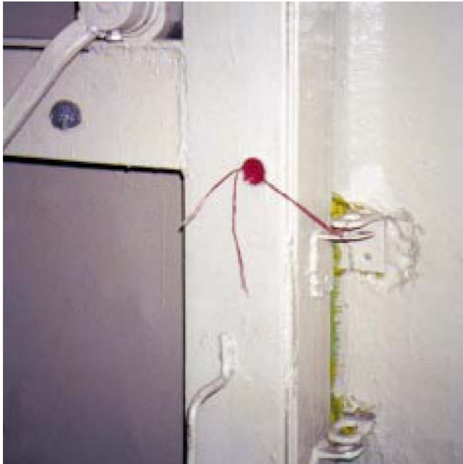
Figure 1. Soviet-era wax and string seal on nuclear material in Russia (From Department of Energy)
