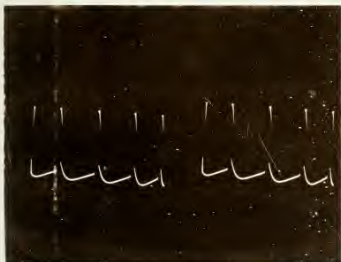
FIG. 10B COLLECTOR VOLTAGE 11 VOLTS PEAK-TO-PEAK
