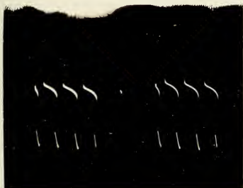
FIG. 10D VOLTAGE OF BASE 13.5 VOLTS PK.-TO-PK.
