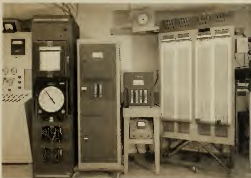
Test Section and Nozzle Block Pressure and Temperature Instrumentation
