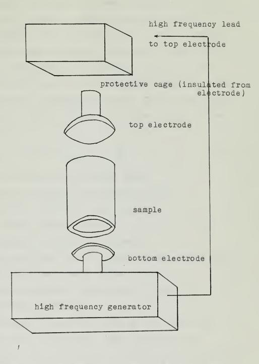
The unit employed in this investigation was a Westinghouse 2 KW dielectric heating unit. The frequency was 27.6 megacycles per second.
