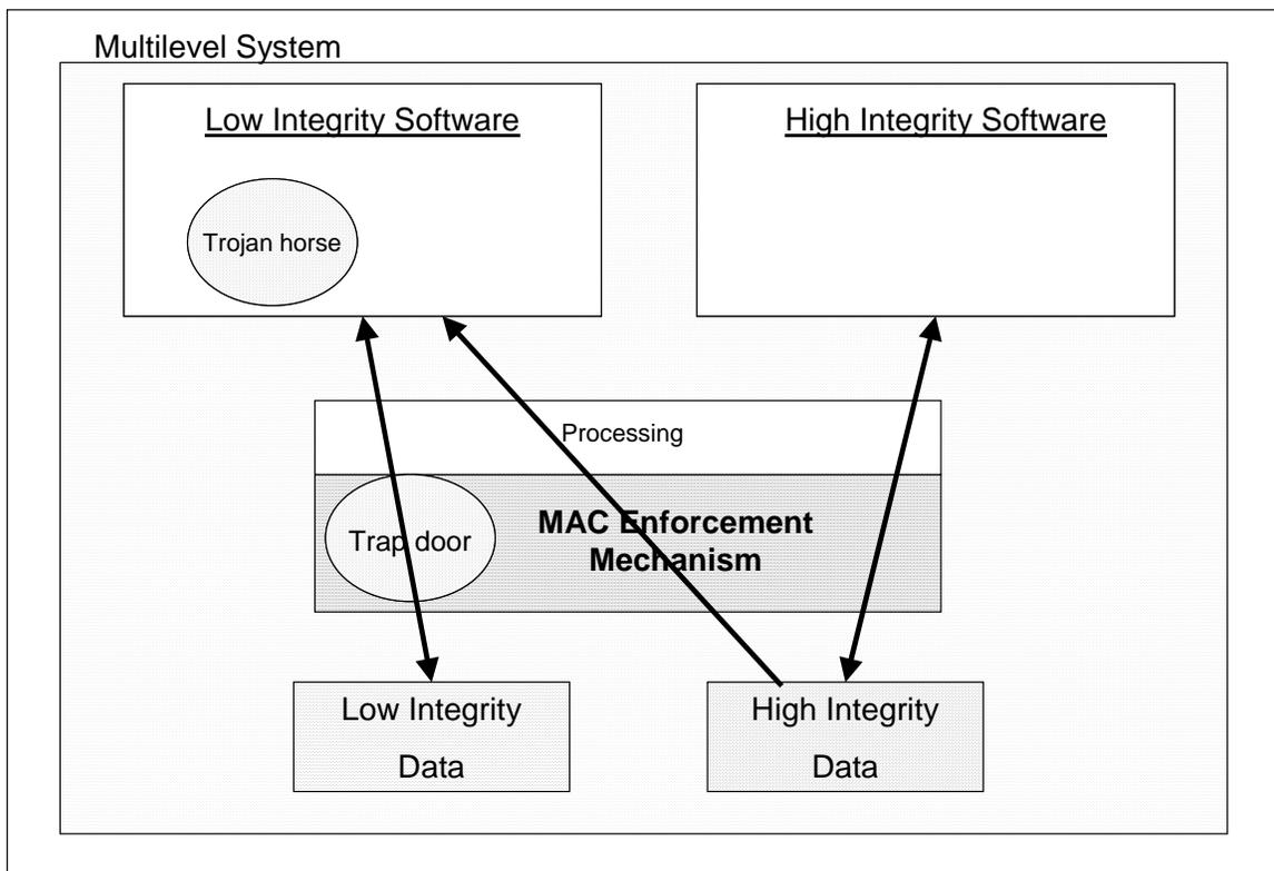
Figure 6. Attack On MAC Enforcement Mechanism
