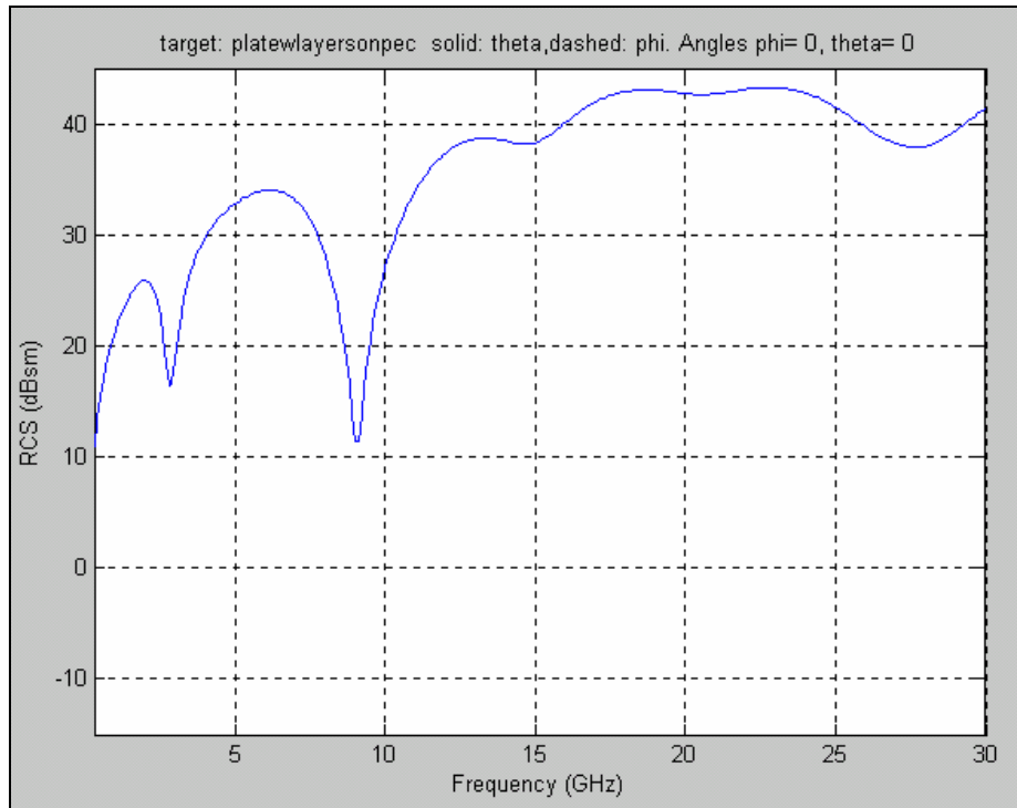
Figure 72. RCS vs. Frequency of a 1 m by 1 m Plate with Two Composite Layers on PEC (normal incidence)
